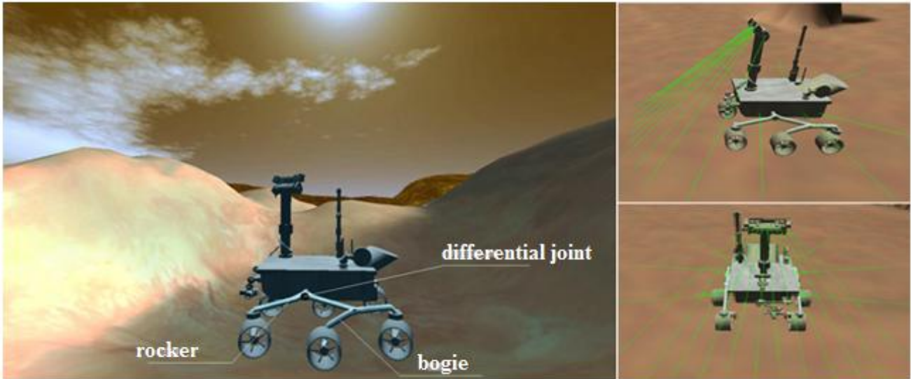
Fig. 1. 3D physics model of the rover highlighting different parts of the rocker-bogie suspension system (left). Side view (top right) and front view (bottom right) of the rover showing lateral and ground sensors and their positions
